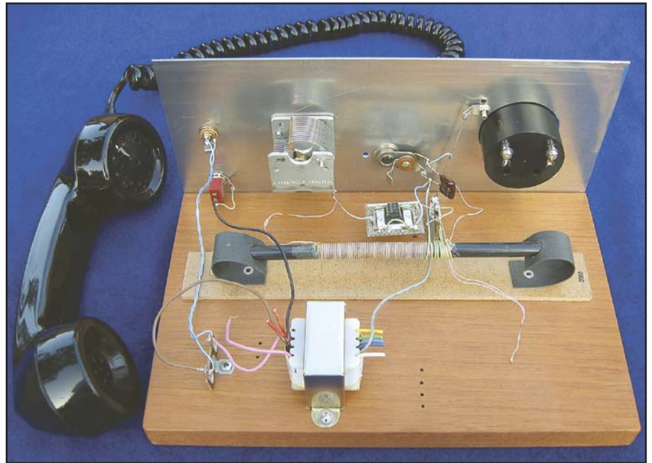
Rear view of the AM band high sensitivity crystal set showing a GTE telephone handset as the headphone. The panel meter is not used for this project.
